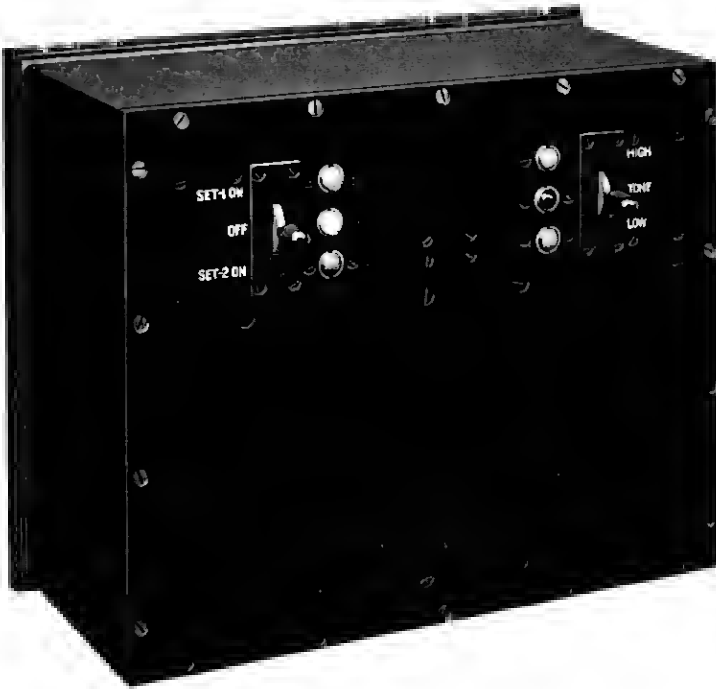
Fig. 6—Control panel for remote control of the monitoring point receivers.
